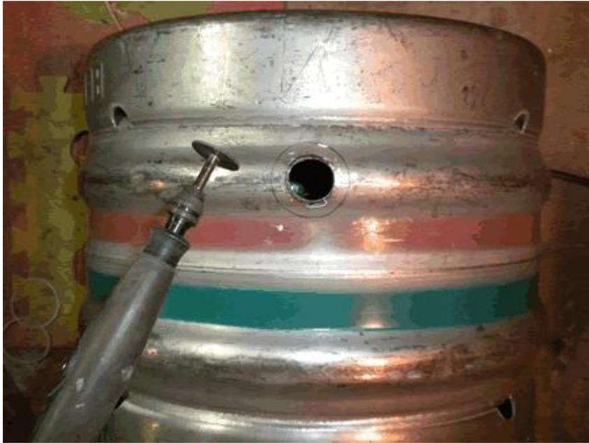
I use my rotary grinder (Dremel, which I am personally finding to be one the most valuable tools for still making) with a grinding disc to enlarge the hole to the exact inside diameter.
