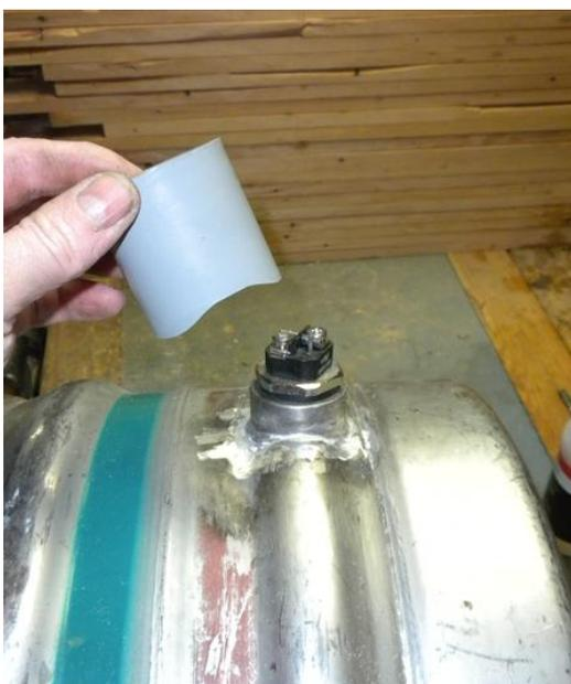
After screwing in my 2000 watt 120V hot water heater element (off the self at any Home Depot) I decided to make the elements electrical connection cover out of a 1 1/2" PVC conduit coupler and a 1 1/2" PVC conduit end cap (again off the self Home Depot).
