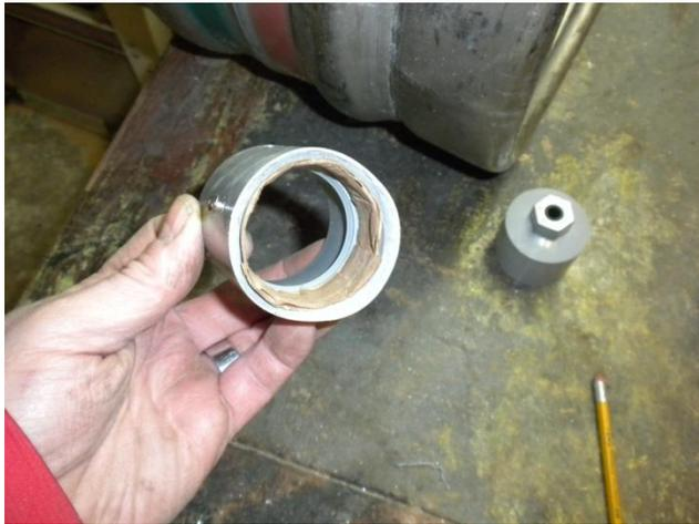
Since the inside diameter of the PVC conduit coupler is just slightly larger than the outside diameter of the stainless steel coupler I used a bit of cardboard to line the PVC coupler to make a very nice tight fit. I
