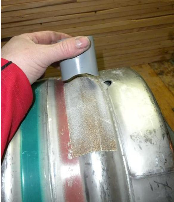
To get the PVC coupler to fit the ridge on the keg I first roughed out the coupler on each side with the rotary grinder and then attached a strip of 60 grit sand paper with some spray glue to the ridge of the keg and moved the coupler over it until it had the perfect contour. I then drilled a 7/8" hole in the top of
