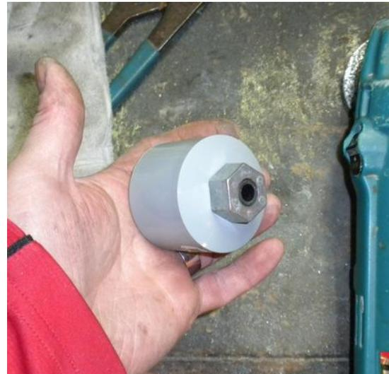
the end cap and ground off the connection end of a 1/2" Cord Grip Connector (Home Depot) which I put through the hole and screwed down the cap to use as the power cord's strain relief.
