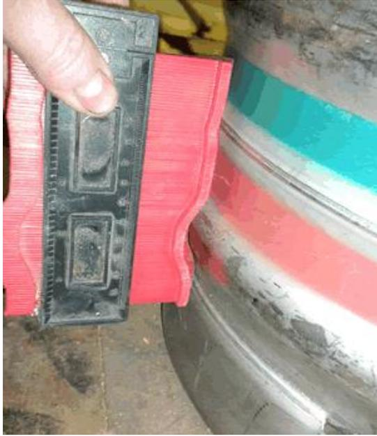
To convert the stainless steel pony keg (7.5 gallons) into a boiler I need to mount a 1" NPT stainless steel half coupler to the side of the keg, (McMaster and Carr part# 4464K475) this will hold most of the off the shelf hot water heater elements that turn the keg into a boiler. I want to solder the 1" NPT half
