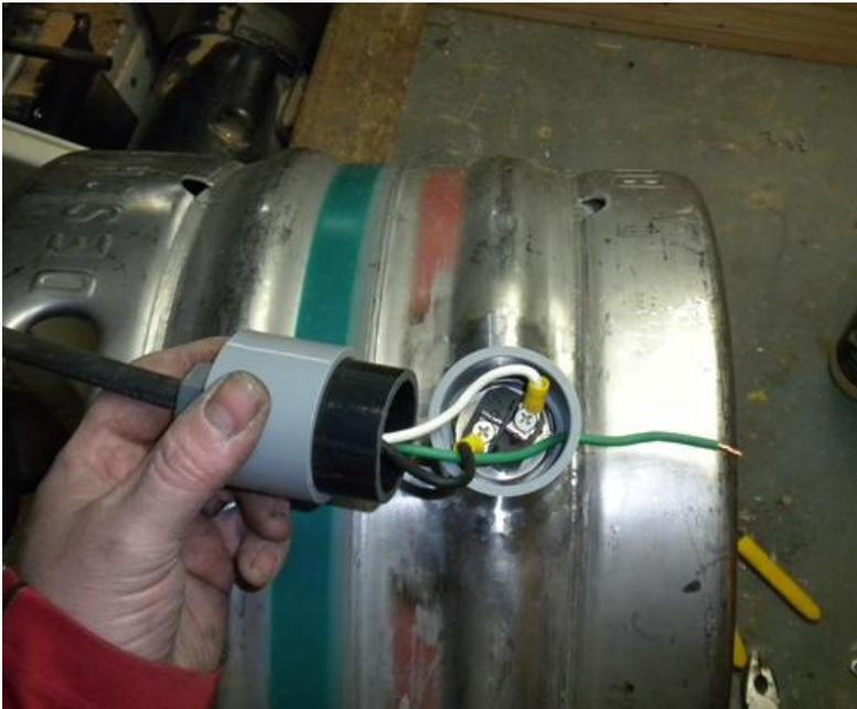
After putting the coupler in place over the stainless steel coupler and hot water heater element I use a short piece of 1 1/2" pipe (maybe 2 1/2" in length) that will join the coupler to the end cap. The wire is
