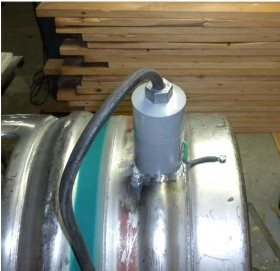
then drilled a hole in the support ring of the keg and tapped the hole for 10-32 threads (you don't need to tap the hole if you use self tapping sheet metal screws). I connect the ground to the keg with a green grounding screw and Ta-Da KEG to Boiler!
