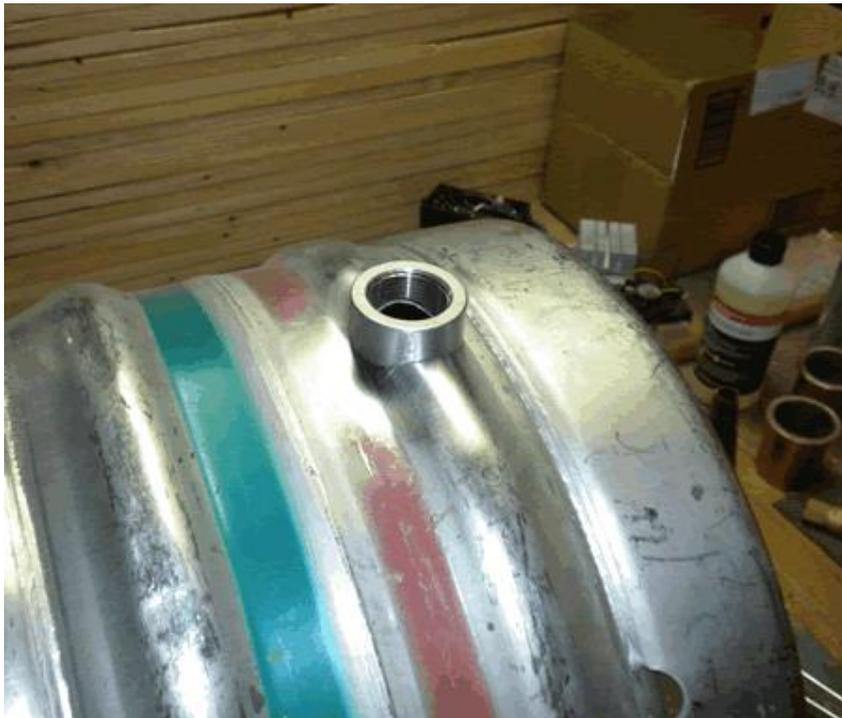
After the keg and coupler are modified I then sand all surfaces until they are smooth and shiny and then further clean with steel wool in preparation for soldering the part together.
