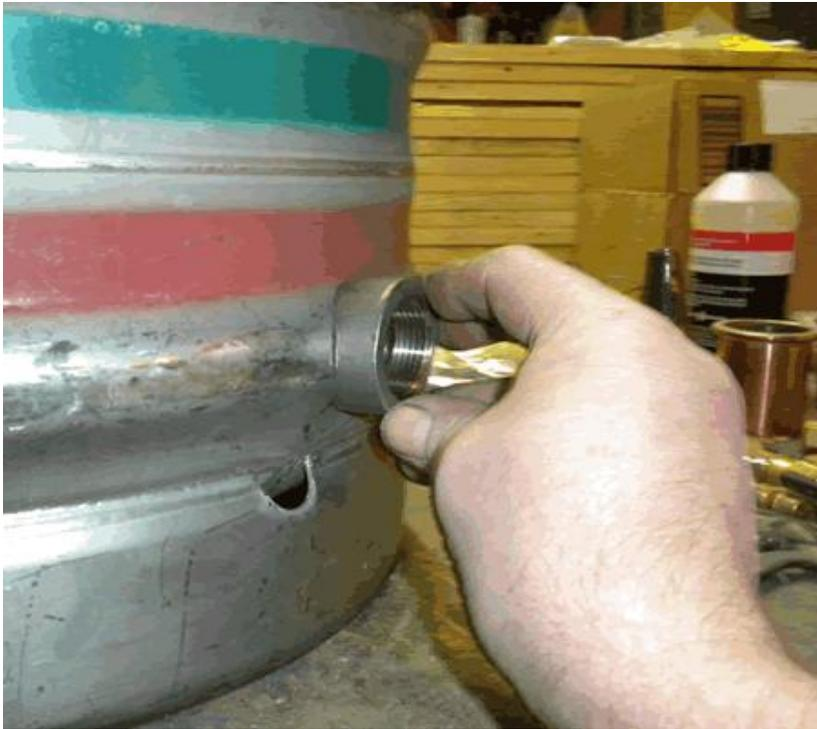
While test fitting the coupler to the keg I use a felt pen to mark the inside and outside diameter of the coupler onto the keg. I then mark the center of the circles and drill a pilot hole (it can be useful to use a punch or even a nail to make a small dent so that the drill bit doesn't travel when starting the hole). I then use a step drill bit to enlarge the hole.
