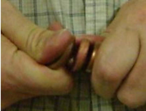
Re-insert mandrel, and use a twisting motion of the screwdriver to evenly space the coil turns (except that last one, at the bottom).
