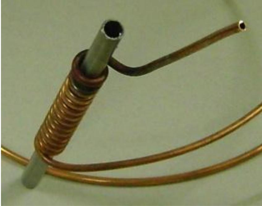
Remove the mandrel and re-anneal the new bend down to the first
