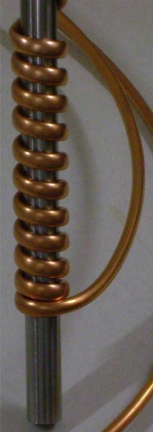
Remove the inner mandrel. You may have to loosen the coil a little by gently twisting it against the direction of the wind. (Hand on left of pic is twisting up, hand on right is twisting down.)
