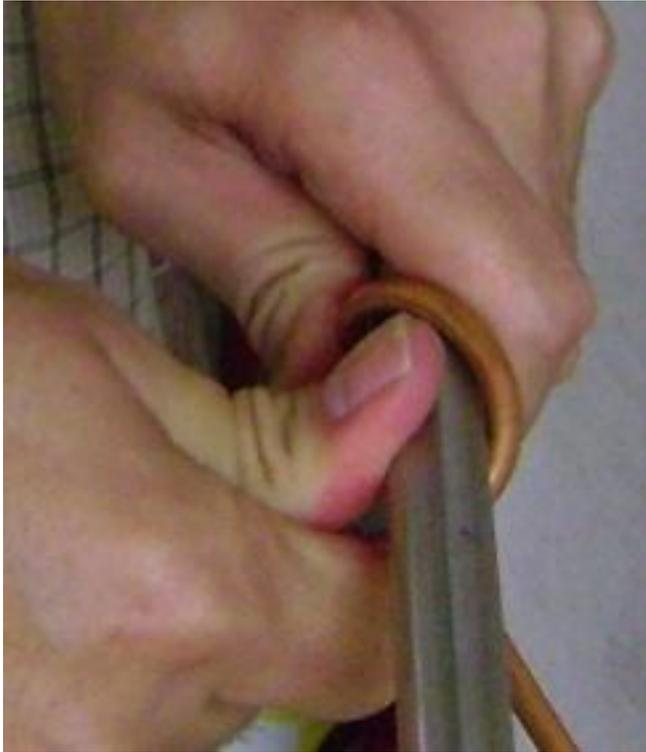
Keep the original angle between the tube and the mandrel until you get most of the way through the first turn, then start changing the angle towards 90 degrees.
