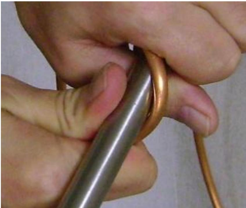
You will get some degree of flattening of the tube as you wind the coils, mainly on the inner coil. This
