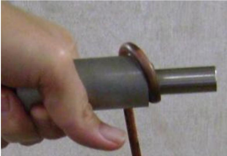
The first turn after getting onto the outer mandrel is difficult, and this is one of the danger points for kinking. But just persist with it a little bit at a time. Try doing this turn in 3-4 steps, rather than all at once.
