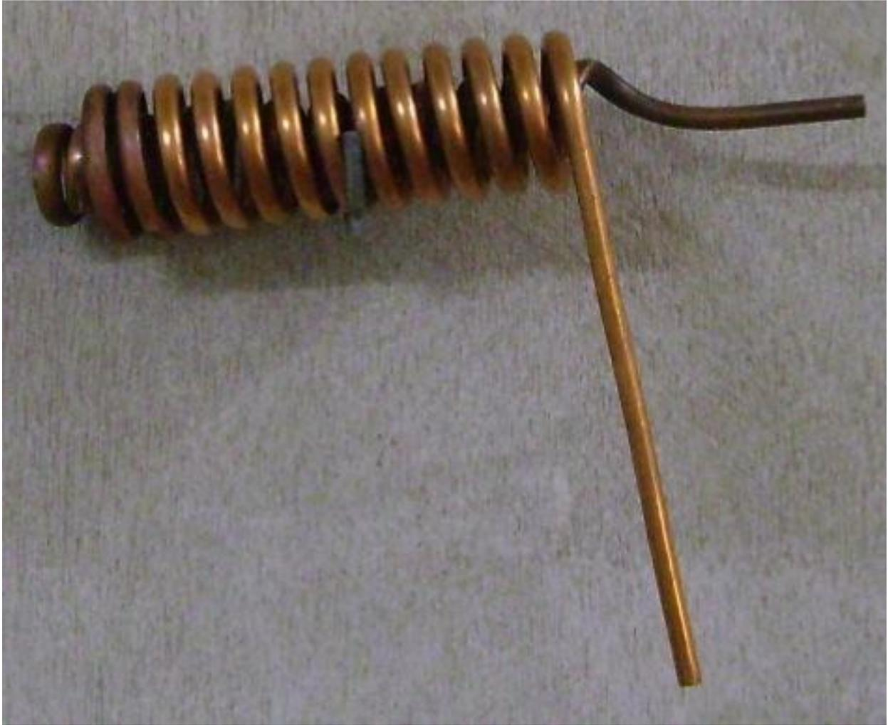
Remove the mandrel and re-anneal the last  $\frac{1}{8}$  of the last turn of the outer coil, and the 40 mm section
