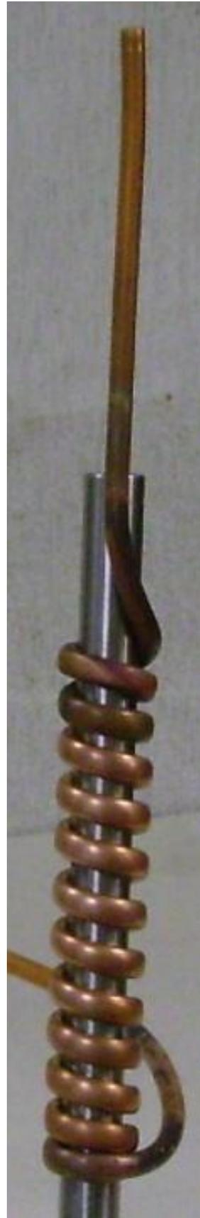
The aim is for the outer mandrel to be able to easily slide over the tail and inner coil.
