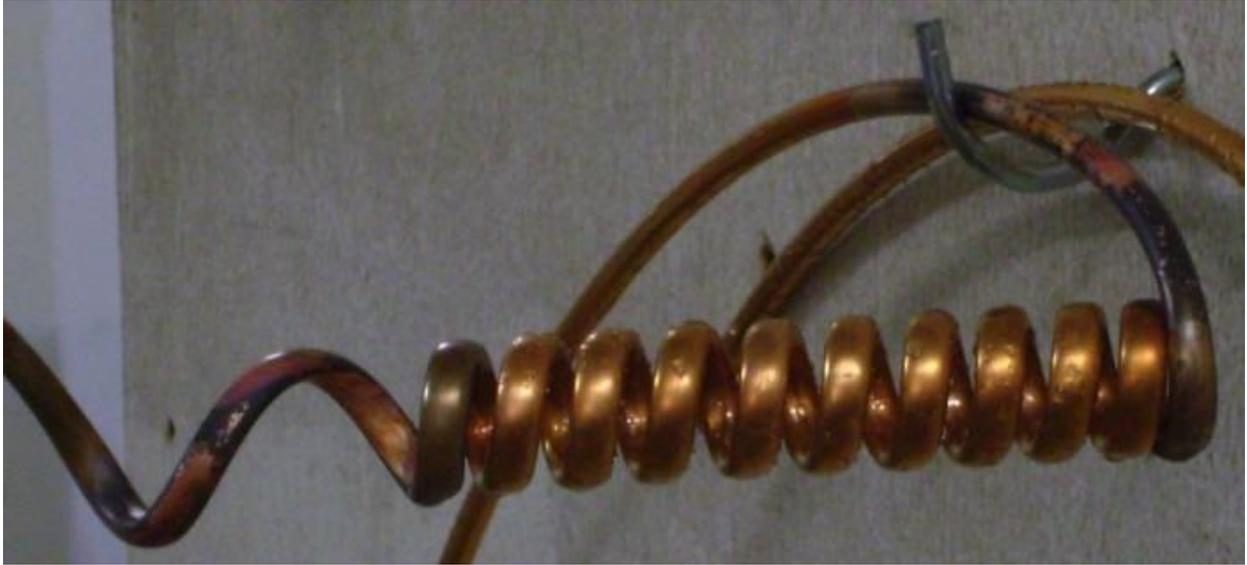
Re-insert the mandrel. Alternatively compress, tighten, and align the widely spaced turn or two at the top of the coil, in steps, and generally work it until it is matched up with the rest of the coil. You may need to re-anneal this section of coil about half way through this process.
