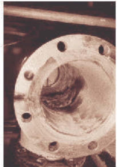
Figure 8. Buildup of scale in the dead end branch of a tee.
